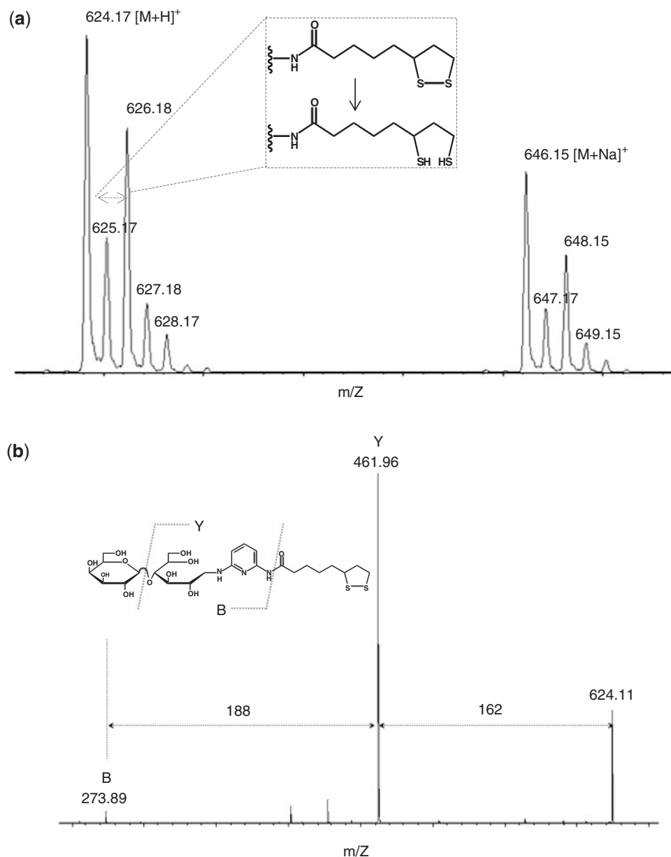
Fig. 2. MS and MS/MS analyses of Gal \beta 1-4Glc-f-mono. A quadrupole ion trap and matrix-assisted laser desorption/ionization time-of-flight mass spectrometer (AXIMA-QIT) was used (see MATERIALS AND METHODS section for details). (a) MS spectrum of Gal \beta 1-4Glc-f-mono; (b) MS/MS analysis of Gal \beta 1-4Glc-f-mono.
